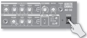
**6.** Switch on any equipment connected to the LINE OUT jack. To turn the power off, reverse these steps.
