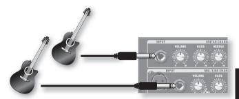
2. Set the [VOLUME] knob of the input you're using to the 5 position (center).
