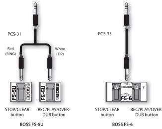
If you've used a cable with a phone plug (mono) to connect only one foot switch, the foot switch will operate only the [REC/PLAY/OVERDUB] button.
