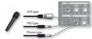
2. Set the [VOLUME] knob of the MIC/LINE CHANNEL to the MIC position.
